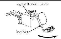
FIGURE 6.13 Installing/Removing Elevating Legrests
